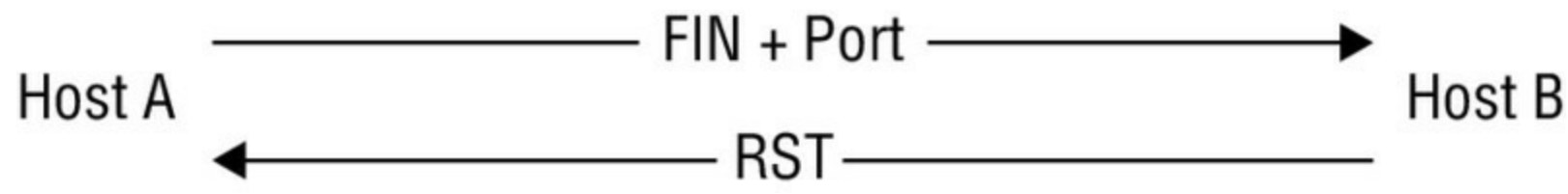
Figure 5.4 An FIN scan against a closed port and an open port
