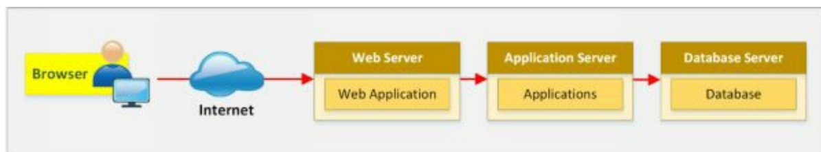
Figure 14-02 Web Application Architecture
