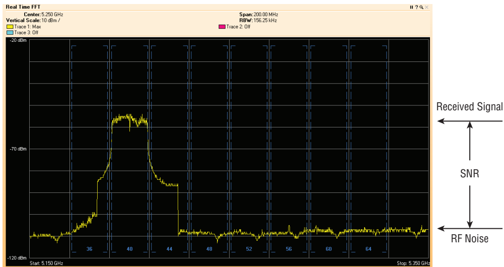
FIGURE 6.23 Graph showing the received signal strength vs. noise floor and the SNR using the Cisco Spectrum Expert spectrum analyzer utility.
