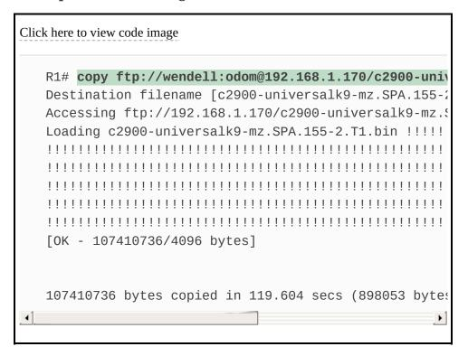
First, take a close look at the long URI in the command that begins with "ftp." The "ftp" part identifies the protocol, of course. After the //, the text references the username (wendell) and password (odom), as well as the FTP server's IP address. After the single / comes the filename on the server.
