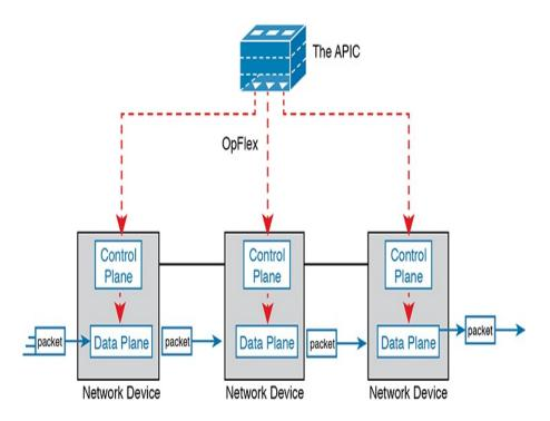
**Figure 16-12** Architectural View of ACI with APIC Pushing Intent to Switch Control Plane
