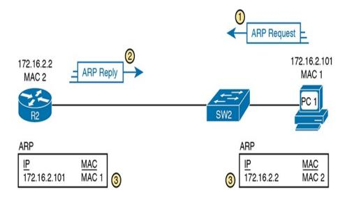
**Figure 8-9** *Legitimate ARP Tables After PC1 DHCP and ARP with Router R2*
