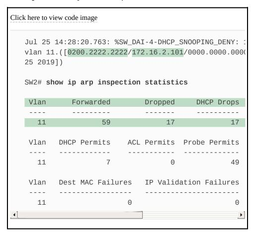
The statistics from the **show ip arp inspection** command also confirms that the switch has dropped some ARP messages. The highlighted lines in the middle of the table show 17 total dropped ARP messages in VLAN 11. That same highlighted line confirms that it dropped all 17 because of the DHCP Snooping binding table ("DHCP Drops"), with zero dropped due to an ARP ACL ("ACL Drops").
