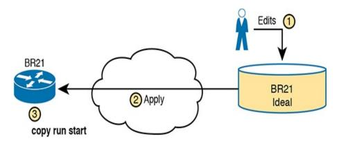
**Figure 19-4** *Pushing Centralized Configuration to a Remote Device*
