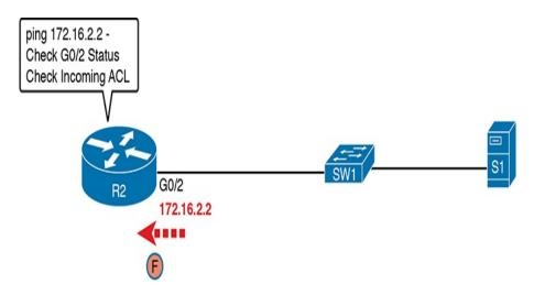
**Figure D-9** *Self-Ping of a Router's Ethernet Address*
