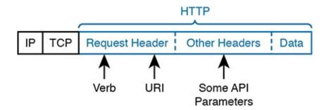
**Figure 18-4** HTTP Verb and URI in an HTTP Request Header
