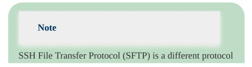
than FTPS. SFTP uses SSH to encrypt file transfers over an SSH connection. However, the acronym SFTP does not refer to a secure version of FTP.
