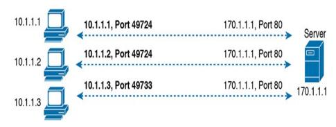
**Figure 10-6** *Three TCP Connections from Three PCs*
