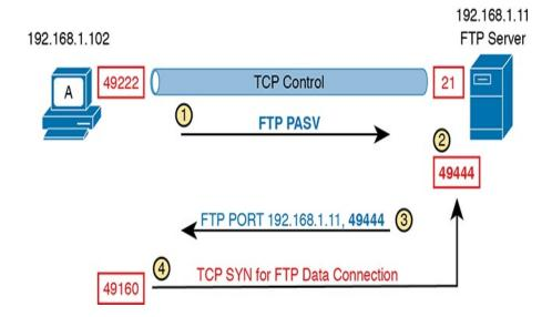
**Figure 12-19** FTP Passive Mode Process to Create the Data Connection
