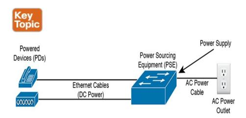
**Figure 13-9** *Power over Ethernet Terminology*
