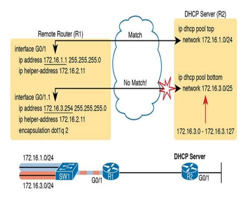
**Figure D-3** An Example Misconfiguration of a DHCP Pool **network** Command
