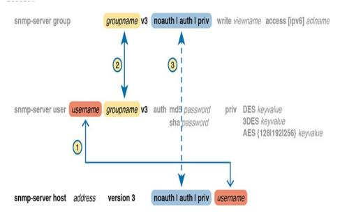
**Figure D-16** Connecting SNMPv3 Notification Configuration with User and Group
