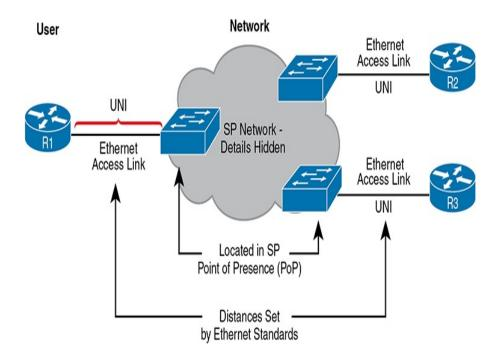
**Figure 14-2** Ethernet Access Links into a Metro Ethernet Service
