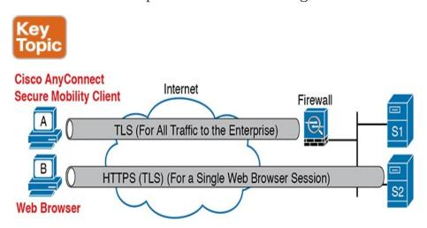
Figure 14-23 Remote Access VPN Options (TLS)
