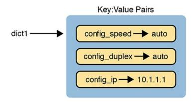
Figure 18-3 Dictionary Data Structures in Python
