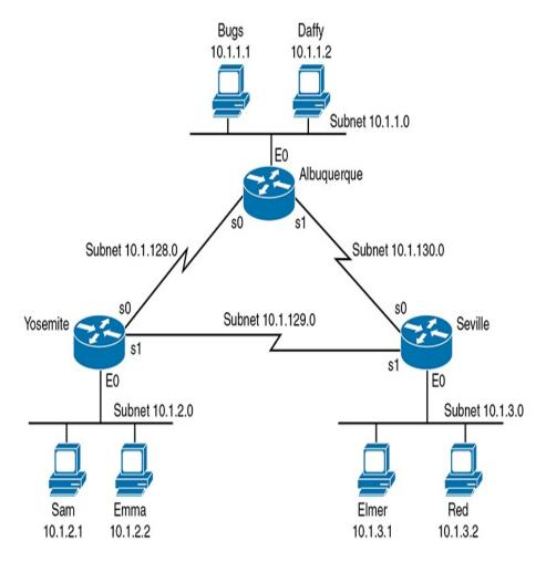
**Figure 3-9** Network Diagram for Extended Access List Example 2
