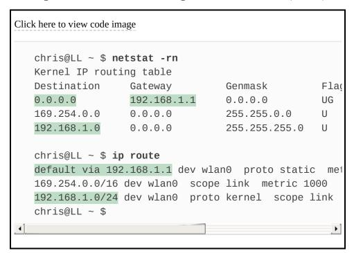
The bottom of the example shows the command meant to replace **netstat -rn: ip route**. Note that it also shows a default
