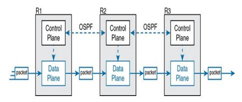
**Figure 16-2** Control and Data Planes of Routers—Conceptual
