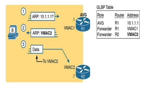
**Figure D-11** *GLBP Directs Host B by Sending Back ARP Reply with R2's VMAC2*
