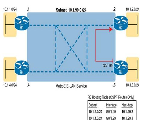
**Figure 14-9** *Layer 3 Forwarding Between Sites with E-LAN Service*
