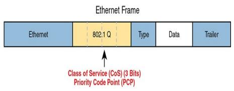
**Figure 11-7** Class of Service Field in 802.1Q/p Header
