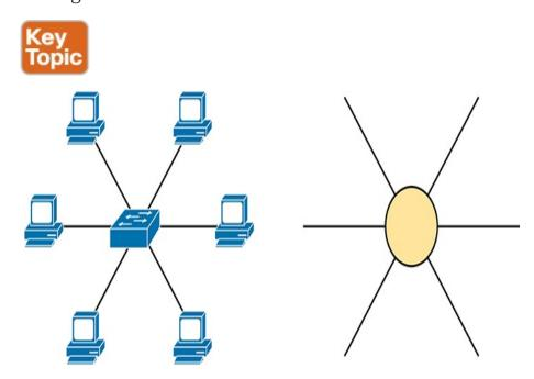
**Figure 13-2** *The Star Topology Design Concept in Networking*
