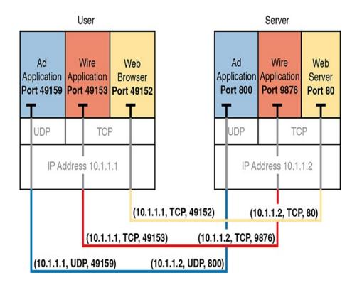
**Figure 1-4** Connections Between Sockets
