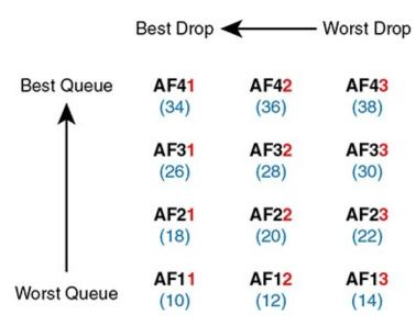
**Figure 11-11** Differentiated Services Assured Forwarding Values and Meaning
