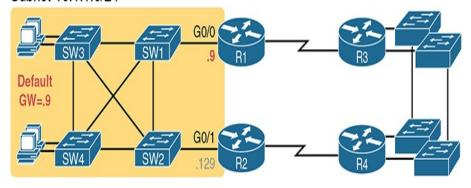
**Figure 12-3** *Removing All Single Points of Failure from the Network Design*
