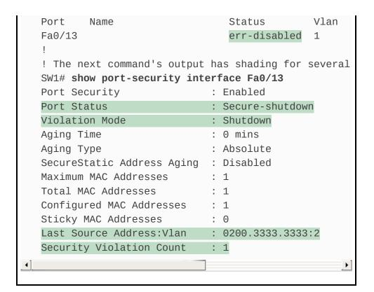
The output of the **show port-security interface** command lists the current port-security status (secure-shutdown) as well as the configured mode (shutdown). The last line of output lists the number of violations that caused the interface to fail to an err-disabled state, while the second-to-last line identifies the MAC address and VLAN of the device that caused the violation.
