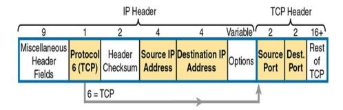
**Figure 11-5** Classification with Five Fields Used by Extended ACLs
