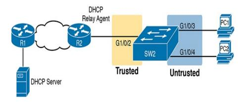
**Figure 8-15** Sample Network Used in ARP Inspection Configuration Examples
