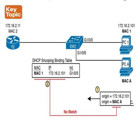
**Figure 8-13** *DAI Filtering ARP Based on DHCP Snooping Binding Table*
