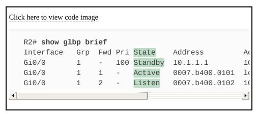
The State column in the output in Examples D-17 and D-18 can pull the GLBP concepts together. First, to define the meaning of the state values, the following short list defines the states expected for the first line of output, about the AVG, and then about each GLBP forwarder:
