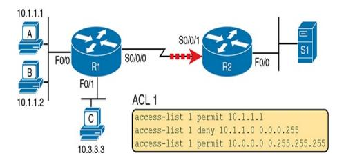
**Figure 2-7** Syntactically Correct ACL Replaces Pseudocode from Figure 2-4
