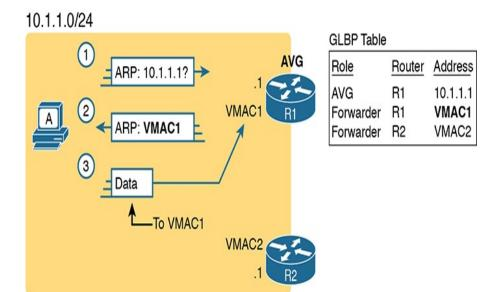
**Figure D-10** *GLBP Directs Host A by Sending Back ARP Reply with R1's VMAC1*
