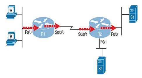
**Figure 2-1** Locations to Filter Packets from Hosts A and B Going Toward Server S1
