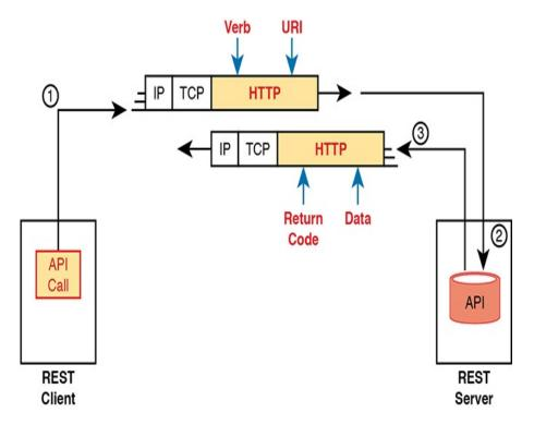
**Figure 18-1** *Client/Server Operation with REST*
