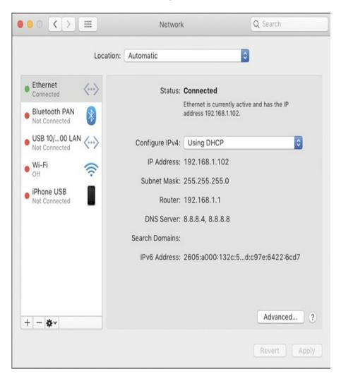
Figure 7-10 IP Address, Mask, and Default Router
