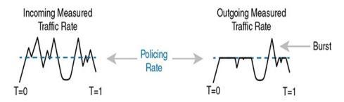
**Figure 11-18** Effect of a Policer and Shaper on an Offered Traffic Load
