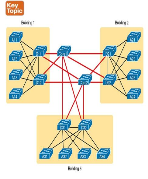
**Figure 13-5** *Three-Tier Building Design (Core Design), Three Buildings*
