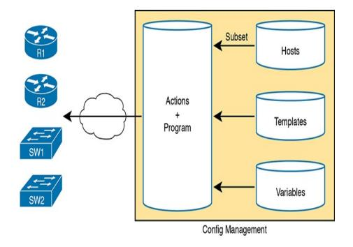
**Figure 19-7** *Important Files Used by Configuration Management Tools*
