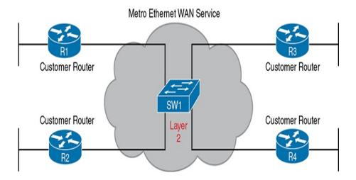
**Figure 14-1** *Metro Ethernet Concept as a Large Ethernet Switch*
