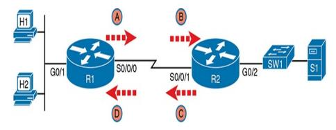
**Figure D-6** Sample Network with IP ACLs in Four Locations
