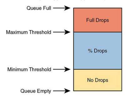
**Figure 11-23** *Mechanisms of Congestion Avoidance*
