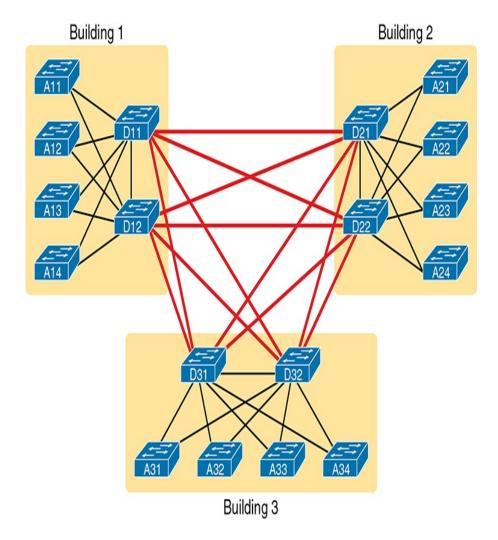
**Figure 13-4** *Two-Tier Building Design, No Core, Three Buildings*
