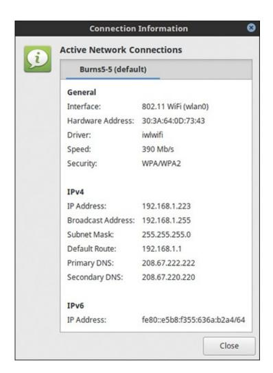
**Figure 7-11** *IP Address, Mask, and Default Router Settings on Linux*
