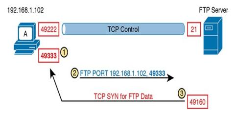
**Figure 12-18** FTP Active Mode Process to Create the Data Connection
