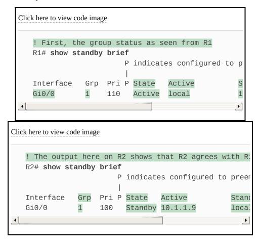
The **show standby brief** command packs a lot of detail in the output, so take your time and work through the highlighted fields. First, look at the Grp column for each command. This lists the HSRP group number, so when looking at output from multiple routers, you need to look at the lines with the same group number to make sure the data relates to that one HSRP group. In this case, both routers have only one group number (1), so it is easy to find the information.
