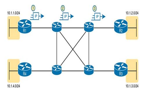
Figure 14-10 Basic IP Routing of IP Packets
