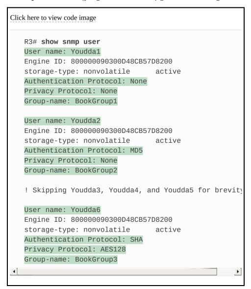
In particular, work through the highlighted output for users Youdda1, Youdda2, and Youdda6, as compared to the configuration in Example D-26. All the highlighted entries basically repeat the settings from the configuration.
