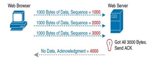
Figure 1-7 TCP Acknowledgment Without Errors
