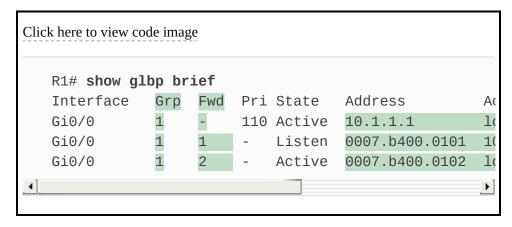
Before looking at the right side of the output, first consider the context for a moment. This example lists a heading line and three rows of data. These data rows are identified by the Grp and Fwd headings, short for Group and Forwarder. With only one GLBP group configured, R1 lists lines only for group 1. More important, each row defines details about a different part of what GLBP does, as follows:
