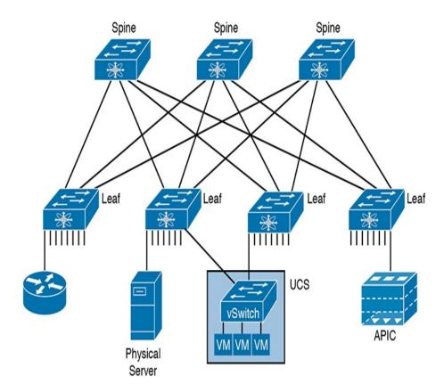
**Figure 16-10** *Endpoints Found on the Leaf Switches Only*
