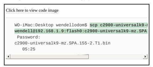
Once you copy the IOS file into a local IOS file system on the router, you must **reload** the router to start using the new IOS. The next topic looks at the entire IOS boot process, including how to make a router start using the new version of IOS.
