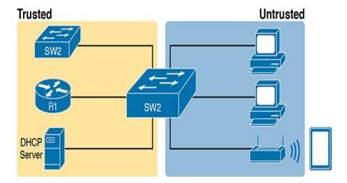
**Figure 8-1** *DHCP Snooping Basics: Client Ports Are Untrusted*
