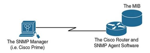
**Figure 12-8** *Elements of Simple Network Management Protocol*
