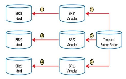
**Figure 19-6** *Concept: Configuration Templates and Variables*
