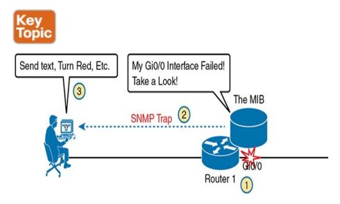
Figure 12-10 SNMP Trap Notification Process
