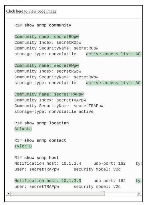
The **show snmp** command takes the opposite approach from the commands in Example D-22, focusing almost completely on status and counter information, rather than repeating configuration settings. This command lists dozens of lines of detailed information, so the sample in Example D-23 shows just enough of the output to give you a sense of the kinds of information found there, with comments following the example.
