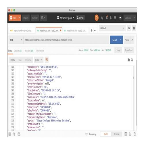
Figure 18-9 URI Structure for REST GET Request
