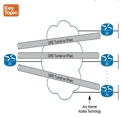
**Figure 14-22** Site-to-Site VPN Tunnels with GRE and IPsec
