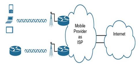
**Figure 14-19** *Wireless Internet Access Using 3G/4G/5G Technology*
