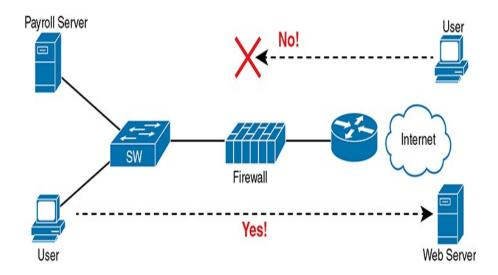
**Figure 5-6** *Allowing Outbound Connections and Preventing Inbound Connections*
