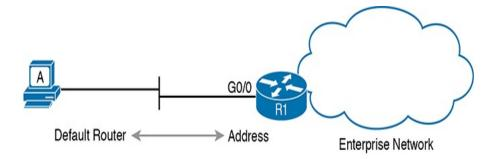
**Figure 7-7** Host Default Router Setting Should Equal Router Interface Address
