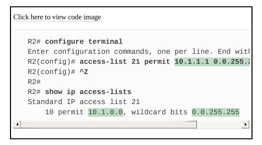
The math to find the range of addresses relies on the fact that either the command is fully correct or that IOS has already set these address octets to 0, as shown in the example.
