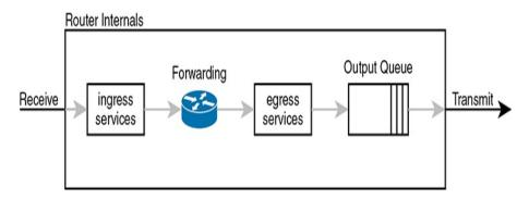
**Figure 11-13** Output Queuing in a Router: Last Output Action Before Transmission
