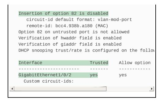
The highlighted lines in the example point out a few of the key configuration settings. Starting at the top, the first two confirm the configuration of the **ip dhcp snooping** and **ip dhcp snooping vlan 11** commands, respectively. Also, the highlighted lines at the bottom of the output show a section that lists trusted ports—in this case, only port G1/0/2.
