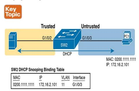
**Figure 8-6** *Legitimate DHCP Client with DHCP Binding Entry Built by DHCP Snooping*
