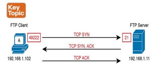
**Figure 12-17** *FTP Client Creates an FTP Control Connection*
