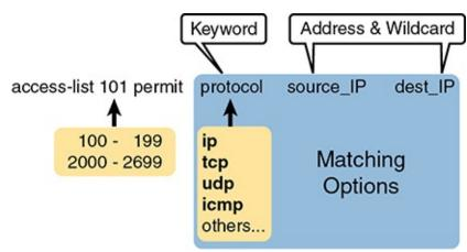
Figure 3-3 Extended ACL Syntax, with Required Fields
