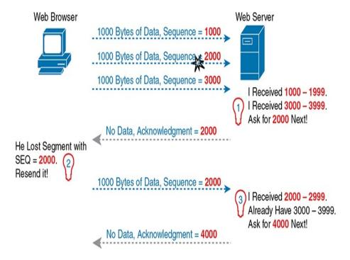
**Figure 1-8** *TCP Acknowledgment with Errors*
