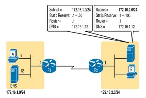
**Figure 7-4** *Preconfiguration on a DHCP Server*
