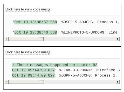
In reality, the messages in both parts of Example 9-6 happened within 0.5 seconds of each other because I issued a **shutdown** command on one of the routers. However, the two routers' time-of-day clocks were not synchronized, which makes the messages on the two routers look unrelated. With synchronized clocks, the two routers would have listed practically identical timestamps of almost the exact same time when these messages occurred, making it much easier to read and correlate messages.
