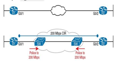
Figure 11-19 Ethernet WAN: Link Speed Versus CIR
