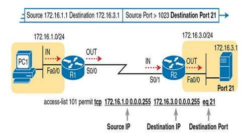
Figure 3-6 Filtering Packets Based on Destination Port
