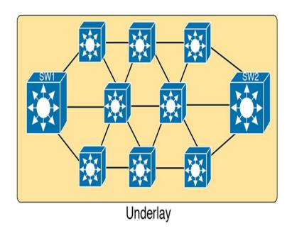
**Figure 17-2** *Fabric, Underlay, and Overlay Concepts*
