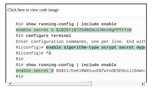
Following the process shown in the example, the first command confirms that the current **enable secret** command uses encoding type 5, meaning it uses MD5. Second, the user
