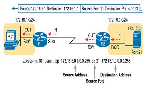
**Figure 3-7** Filtering Packets Based on Source Port
