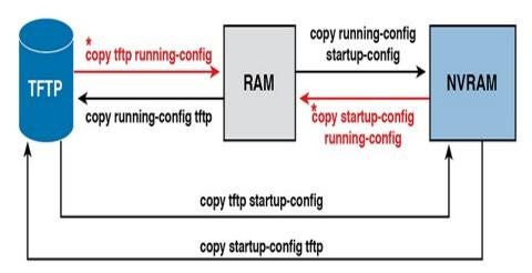
**Figure F-5** Copy into RAM (running-config) Adds Configuration Instead of Replacing
