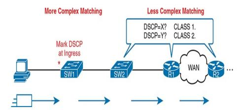
**Figure 11-4** *Systematic Classification and Marking for the Enterprise*
