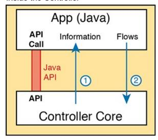
**Figure 16-6** *Java API: Java Applications Communicates* with Controller
