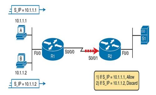
**Figure 2-2** Pseudocode to Demonstrate ACL Command-Matching Logic
