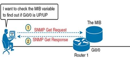
**Figure 12-9** *SNMP Get Request and Get Response Message Flow*
