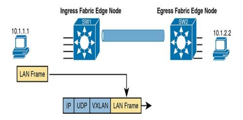
**Figure 17-5** Fundamentals of VXLAN Encapsulation in SDA
