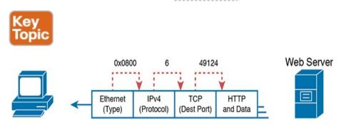
**Figure 1-16** Three Key Fields with Which to Identify the Next Header
