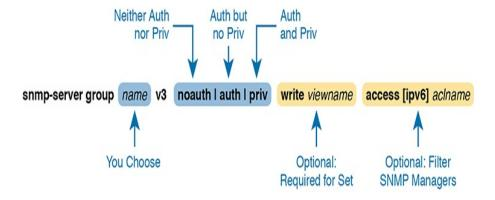
**Figure D-13** *SNMPv3 Groups—Configuration Command Parameters*
