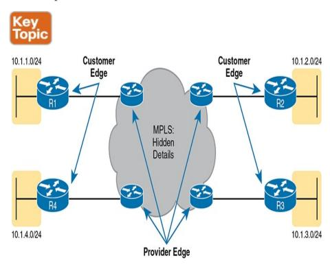
**Figure 14-11** *MPLS Layer 3 Design*, with *PE and CE Routers*
