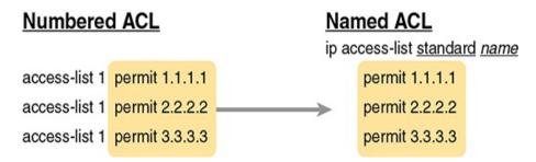
**Figure 3-10** Named ACL Versus Numbered ACL Configuration
