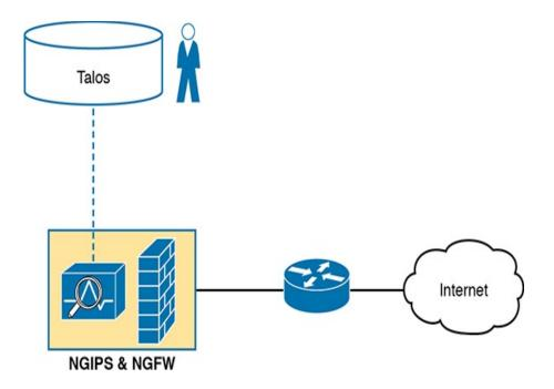
**Figure 5-10** *Next-Generation Firewall with Next-Generation IPS Module*
