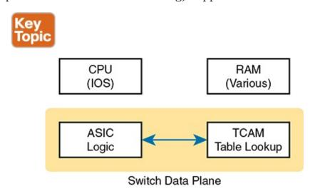
**Figure 16-4** *Key Internal Processing Points in a Typical Switch*
