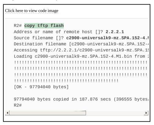
The **copy** command does a simple task—copy a file—but the command also has several small items to check. It needs a few pieces of information from the user, so the command prompts the user for that information by showing the user some text and waiting for the user's input. The bold items in the example
