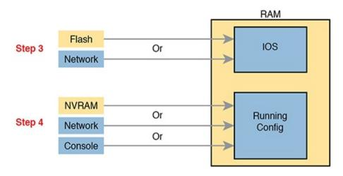
Figure F-3 Loading IOS and Initial Configuration
