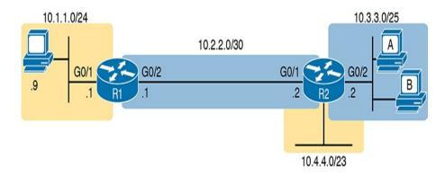
**Figure D-5** Example Network Used in IPv4 ACL Troubleshooting Examples
