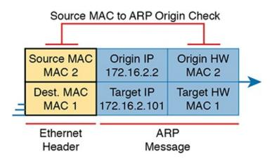
**Figure 8-14** *DAI Filtering Checks for Source MAC Addresses*
