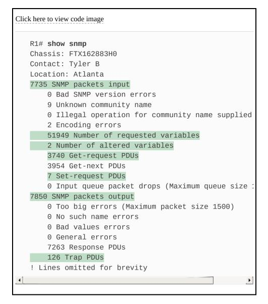
The output in Example D-23 was taken from Router R1 as shown in the earlier examples, after doing some testing from the NMS at address 10.1.3.3. The highlighted items point out
