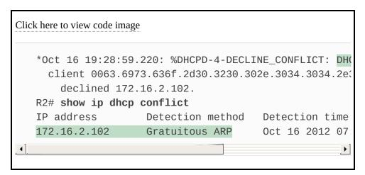
The **show ip dhcp conflict** command lists the method through which the server added each address to the conflict list: either gratuitous ARP, as detected by the client, or ping, as detected by the server. The server avoids offering these conflicted addresses to any future clients, until the engineer uses the **clear ip dhcp conflict** command to clear the list.
