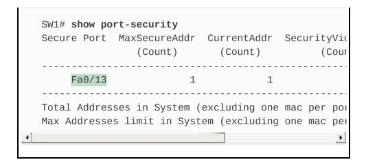
Note that for these next examples, a switch has configured port security on port Fa0/13 only. In this case, the switch appears to be configured to support one MAC address, has already reached that total, and has a security violation action of "shutdown."
