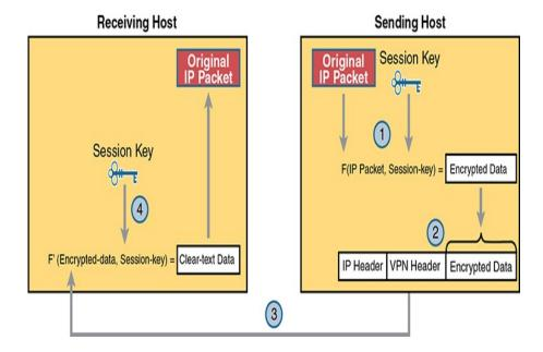
Figure 14-21 Basic IPsec Encryption Process
