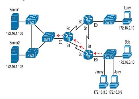
**Figure 3-8** Network Diagram for Extended Access List Example 1
